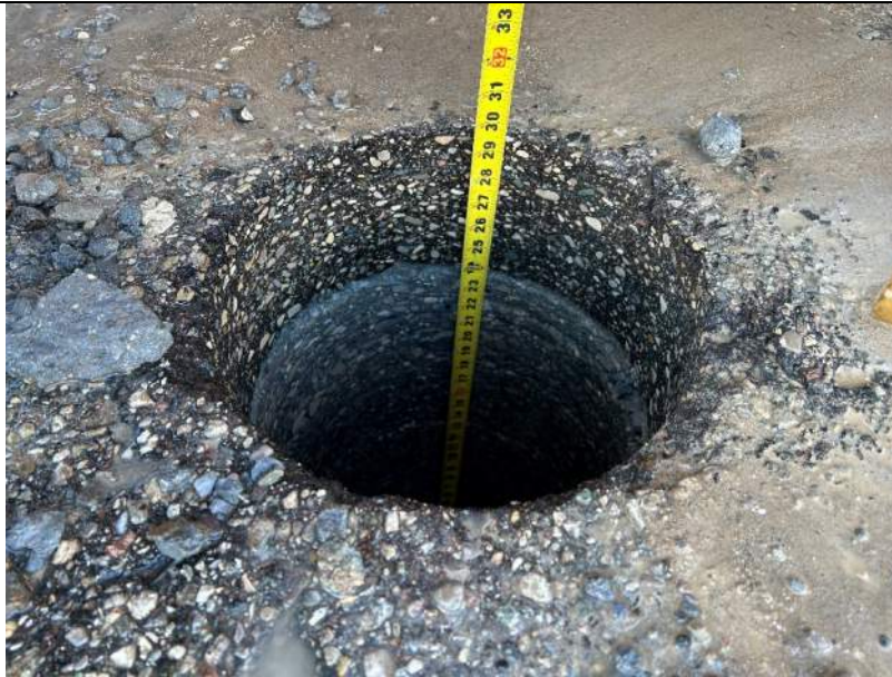
Photo No. 5 – Image Showing Thickness of HMA and RCC Layers
